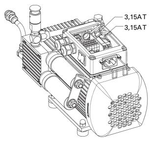
Fig. 5: Replacing the fuses
